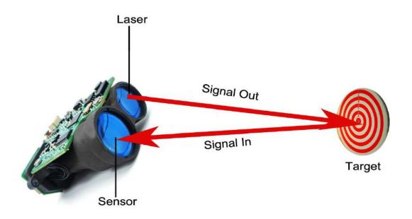
The laser reflected by the measured target passes through the receiving antenna of the optical system and converges to the photodetector, where it is converted into an electrical signal. The control and information processing circuit processes the transmitted laser pulse signal and the echo laser pulse signal to obtain the distance information of the measured target, which is transmitted to the host computer through the communication interface to complete the laser ranging.
